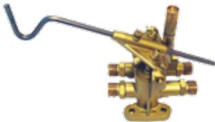
Considerable savings in gas costs can be achieved by the use of a gas economiser in production welding and brazing. The torch is held on the hooked arm when not in use which shuts off gas supply to the torch. When unhooked the torch can be immediately re-ignited from the pilot light without having to re-adjust the valves. 3/8" BSP connections.
