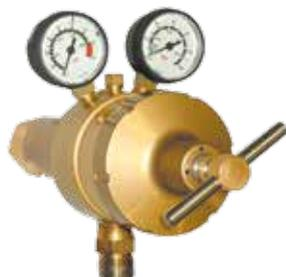
"S1510L2" SERIES – this pipeline regulator is ideal for tank systems, rear entry to suit panel or line mounting. The large outlet configuration is necessary to give high flow from a relatively low inlet pressure source. Max inlet 24 bar and delivery up to 10 bar.
