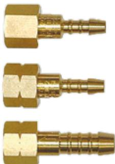
Hose check valves prevent the reverse flow of gases beyond the torch inlets. GCE hose check valves are manufactured to our own approved design and the unique method of assembly eliminates the use of soldered or bonded joints. They are suitable to use with Oxygen, Acetylene, Propane or Natural Gas and operate effectively on either nozzle mix or injector type torches or machine cutting torches.
